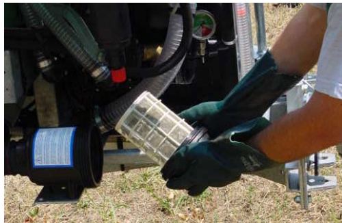
Dismantling the Suction Filter
